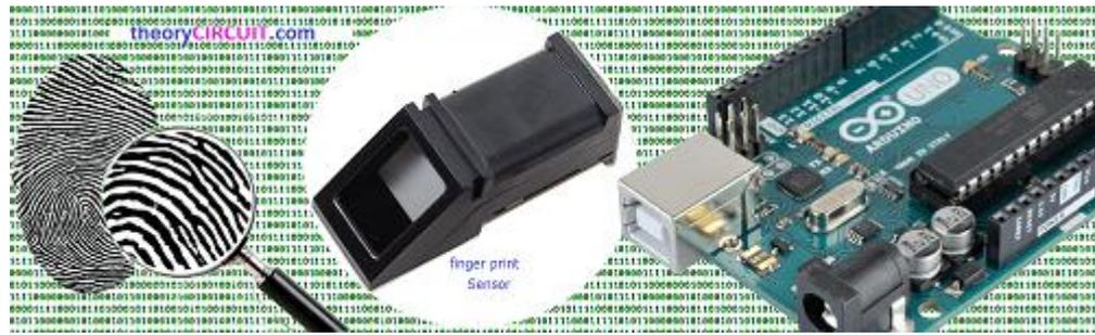
The Fingerprint is one of the safest way to detect and identify the Authorized person, We know that fingerprint is unique even identical twins do not have identical fingerprints. By using this we can make pretty sure about security needs. To add fingerprint verification in microcontroller projects we can use this all in one optical fingerprint sensor-scanner (R305), It makes fingerprint detection and verification super simple.
