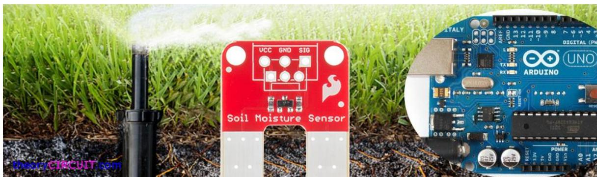
Want to know and data log the moisture level of soil, here is the sensor to do so, the moisture sensor has two large exposed pads function as probes for the sensor and together acting as a variable resistor. Put the sensor into the soil where you want to measure moisture level depends on the water presence in the soil the sensor's conductivity between the pads will vary that is more water more conductivity.
